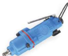
OP-309B 3/8" Side exhaust 側排氣
