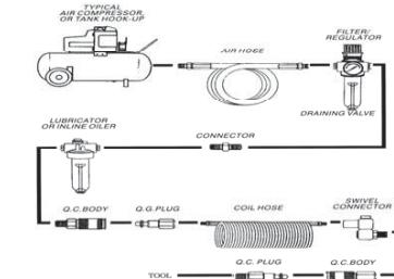
2.2 Before connecting the air hose, please apply 4 to 5 drops spindle oil(M12) at the air inlet. Moreover, oiling is necessary after operating 3 to 4 hours.
